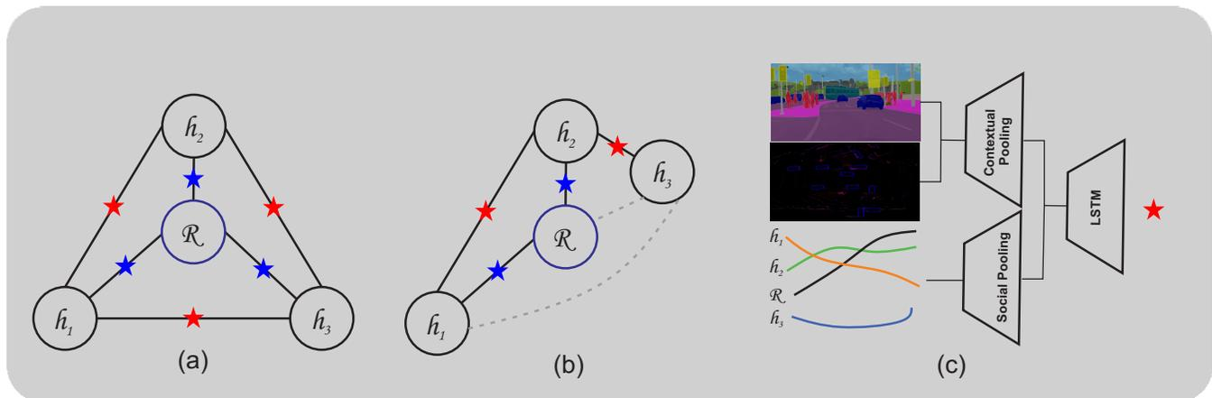
**Figure 1: a: proposed factor graph, red star for factor of human-human interaction, blue star for factor of human-robot interaction, b: factor graph after elimination, c: considered feature extraction to model the social interaction, above: semantic grid, middle: navigation grid, below: trajectories**
